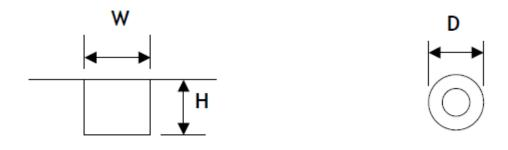
Typical groove design for circular profile gaskets -
