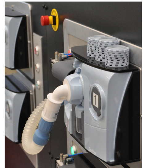
Nolato MediTor injection-molds nine components in plastic, TPE and silicone. These are assembled on a semi-automated line and undergo thorough inspection before being packaged and supplied direct to Dräger’s customers in the healthcare sector.
